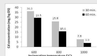
Effect of temperature and time on Cd concentration within soil;
