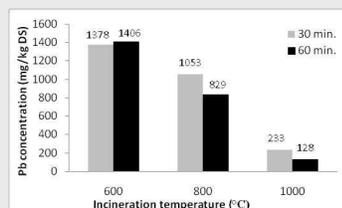
Effect of temperature and time on Pb concentration within soil;
