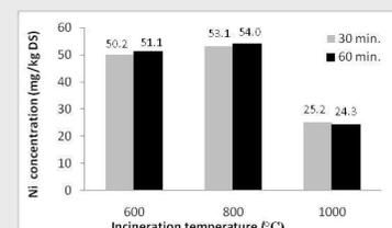
Effect of temperature and time on Ni concentration within soil;
